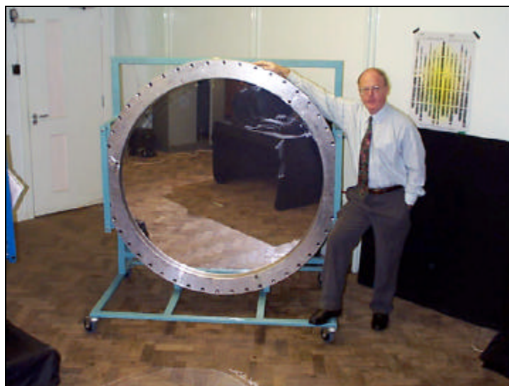
Figure 1: 1.2-m diameter stretchable membrane mirror.
