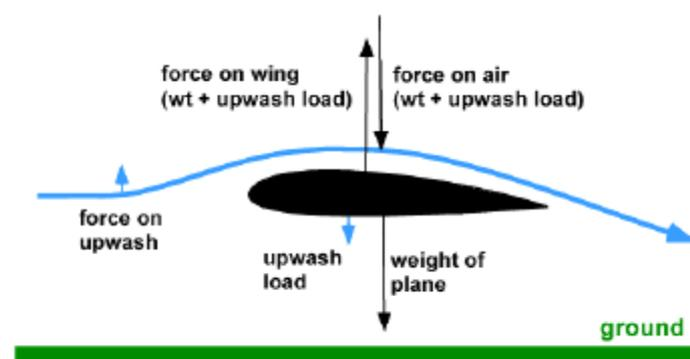
Fig 16 Wing in ground effect
