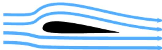
Fig 2 Common depiction of airflow over a wing. This wing has no lift.
