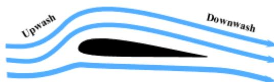
Fig 3 True airflow over a wing with lift, showing upwash and downwash.
