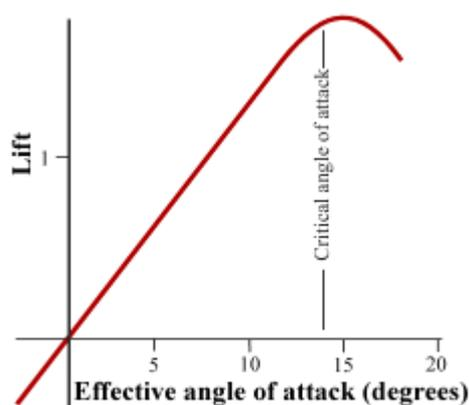
Fig 8 Lift versus the effective angle of attack.
