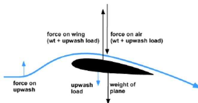
Fig 15 Wing out of ground effect
