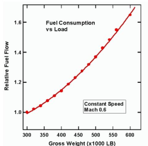
Fig 12 Fuel consumption versus load for a large transport airplane traveling at a constant speed.
